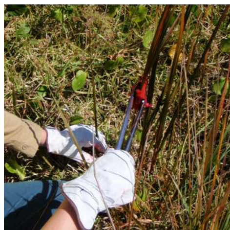
A specially designed hand-held tong-like herbicide applicator called by the control team “Tongs of Death”. The tongs are used to apply herbicide directly to the Watsonia leaves in a manner similar to a wick applicator.
