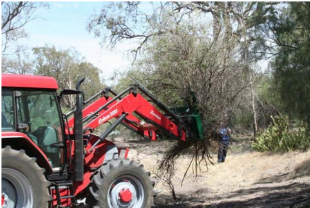
African boxthorn puller in action. Image: New South Wales National Parks & Wildlife Service.
