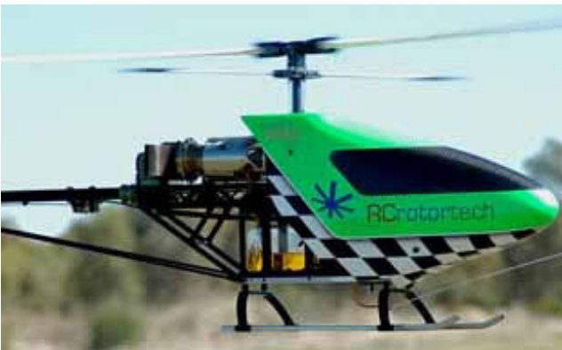
The Zealous II radio-controlled scale turbine helicopter will be fitted with a sensitive imaging system to detect weed distribution.
