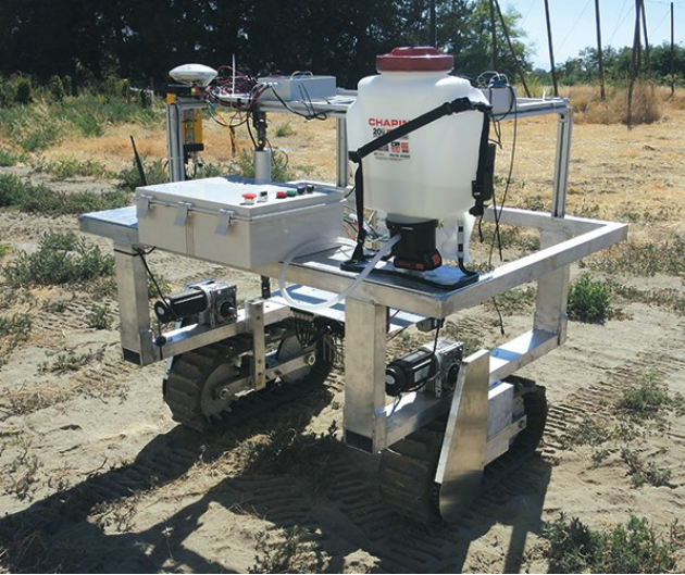
A robotic weeder was developed for the onion industry and has ability to spray weeds Image: Onion world
